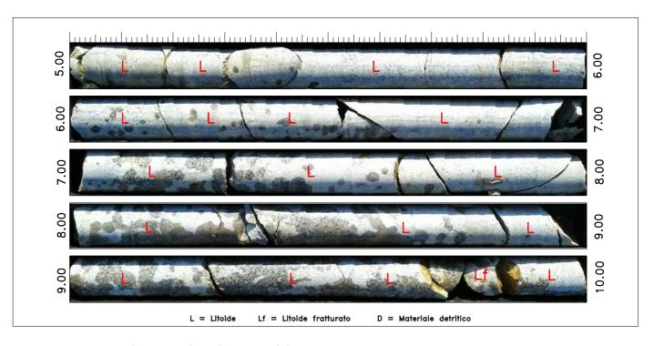
R.Q.D.(5.00-6.00) = (27+39+16)/100\*100 = 82% Buono R.Q.D.(6.00-7.00) = (51+34)/100\*100 = 85% Buono R.Q.D.(7.00-8.00) = (28+30+36)/100\*100 = 94% Eccellente R.Q.D.(8.00-9.00) = (32+56)/100\*100 = 88% Buono R.Q.D.(9.00-10.00) = (27+41+14)/100\*100 = 82% Buono
